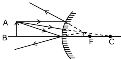
Same orientation so image is virtual. It is combination of real object and virtual image using height it is possible only from convex mirror.
